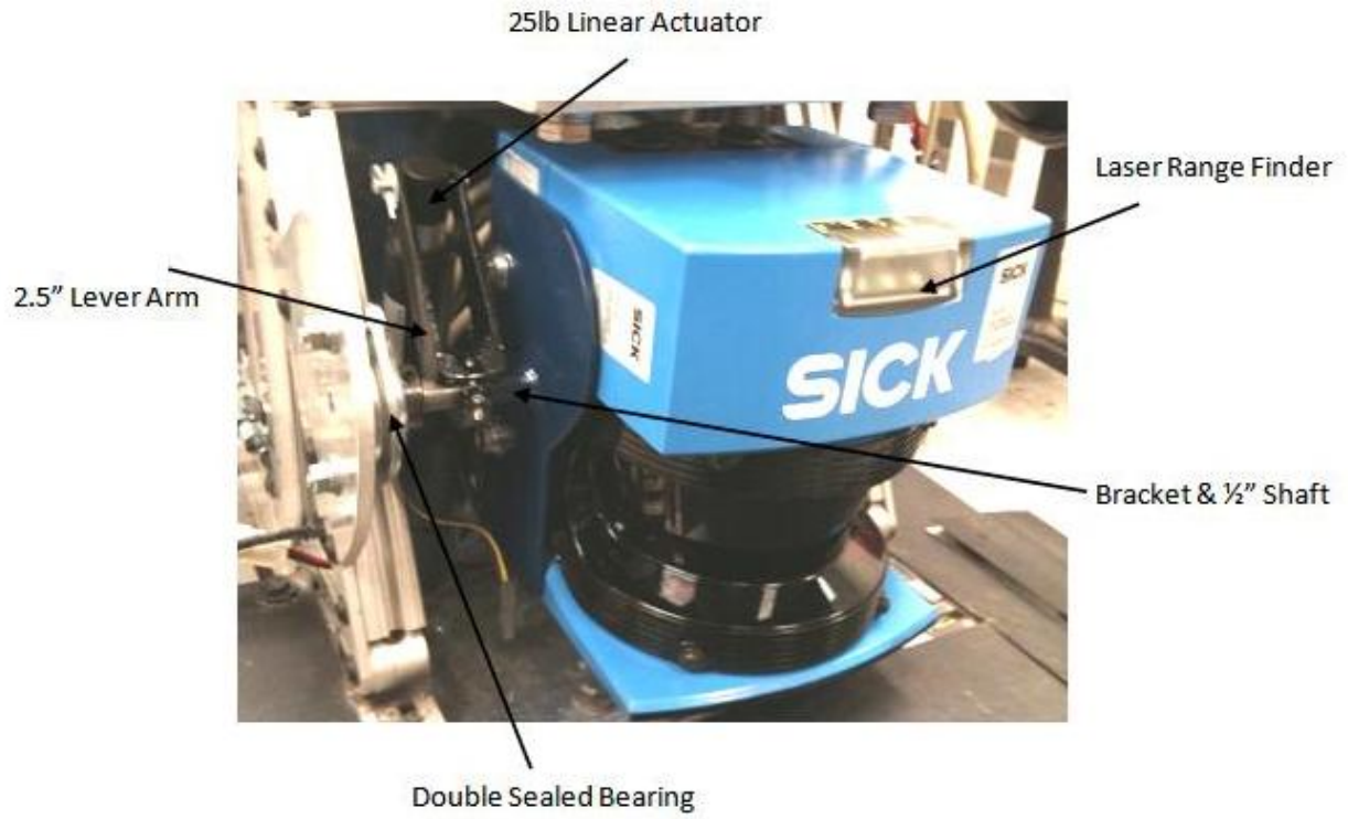
Figure 4: Linear Actuator and Laser Range-Finder [1]
