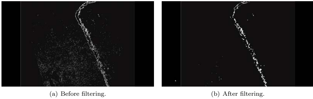
Figure 17: The results of post processing using morphological opening and median filtering. As can be seen, the results in 16(b) have much less noise.
