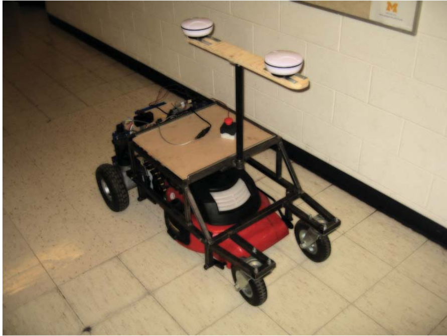
Figure 8: AGM after electronics tray was installed.
