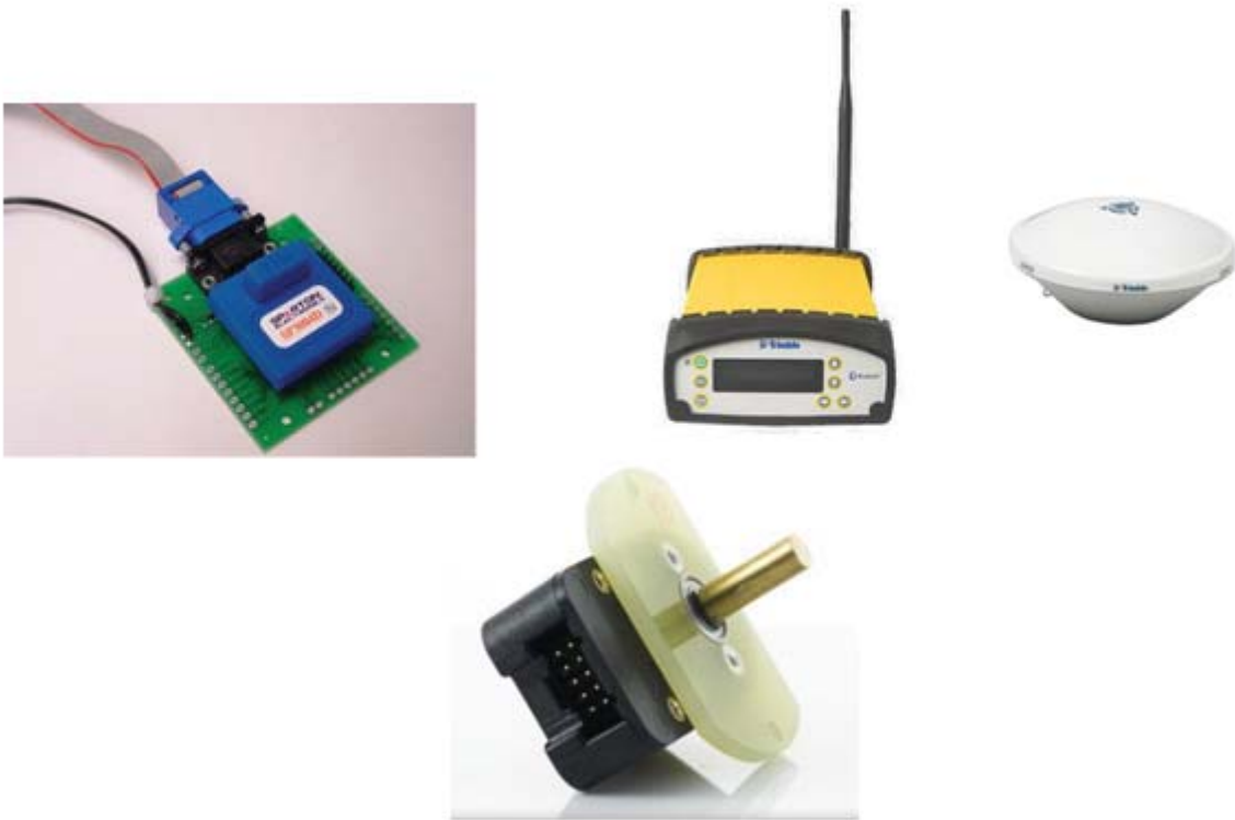
Figure 23: Navigation Subsystem Components (From left to right, digital compass, DGPS and digital encoder)
